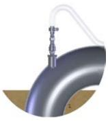
The nozzle unit is welded to the dropleg and Nopon Cleans' feeding hose is attached to the nozzle unit with a quick-release fitting.
